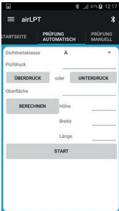
In the Surface field the surface area can be set between 0,1 and 2,000 m<sup>2</sup>.
