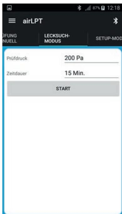
A test duration of 1 to 30 minutes can be set in the DURATION field (the default time on opening this mode is 15 minutes).
