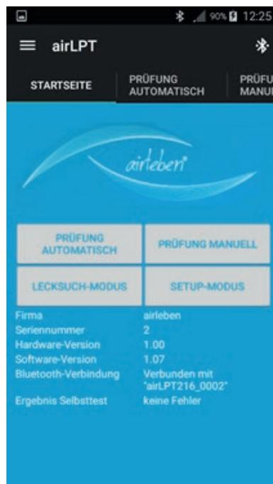
The device details such as company name, name of the device, hardware version, software version and the status of the self-test are read out and displayed.
