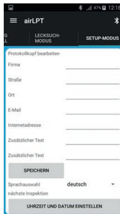
The device data are read out and displayed in the app. The record header data are displayed and can be changed. After pressing the Save button the data is transmitted to the tester.
