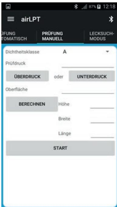
This corresponds to automatic test mode, with the exception that the test pressure must be adjusted manually by changing the fan speed to the entered target value.
